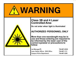
Unattended Laser in Operation, Class 3B or Class 4 must be identified with warning sign when the exterior boundry of a non-interlocked laser use area that contains unattended open beams is in operation. Temporary Laser Controlled Areas for Class 3B and Class 4 laser systems must have appropriate NOTICE signs. Examples:
