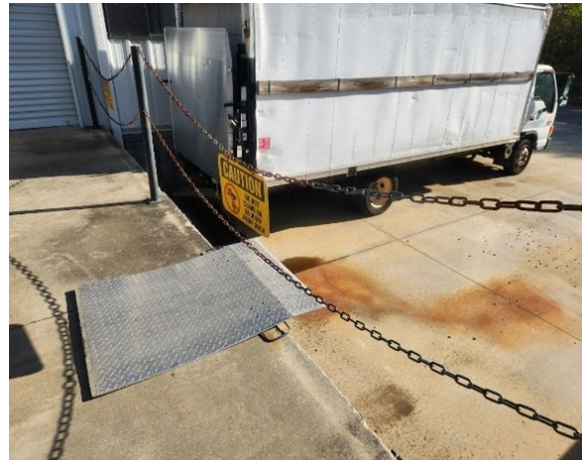
Portable Dock Plate And Chain Guard In Place
